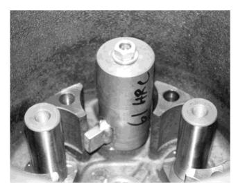
**Picture 5.** Planet gear shafts removing with a special tool.
