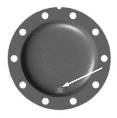
Picture 1. Wheel hub drain plug.
