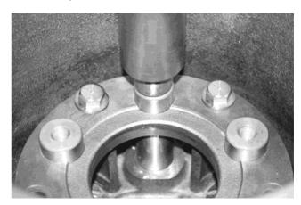
Picture 10. Installation the planet gear shafts.
