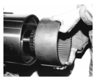
**Picture 7.** Removing the ring gear and the ring gear hub.
