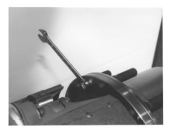
Picture 2. Unscrewing hub housing retaining screws.
