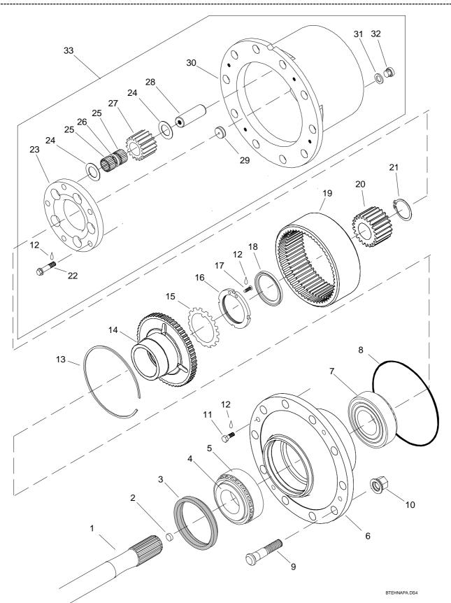
Picture 9. Exploded view of wheel hub assembly.
