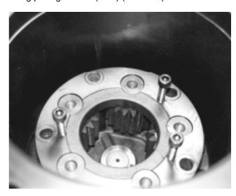
**Picture 4.** Using planet carrier pulling screws.
