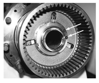
Picture 6. Bearing adjustment nut lock screws.
