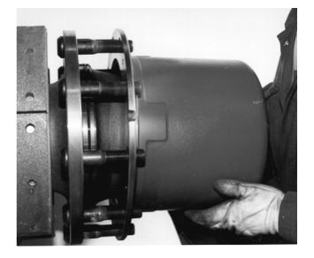
Picture 3. Hub housing removal.
