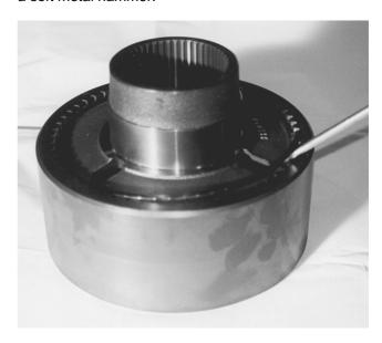
Picture 8. Retaining ring removal.
