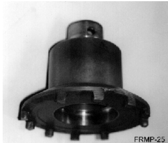
Picture 35: Special tool for the adjustment nut
