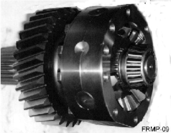
Picture 11: Input shaft complete with related parts
