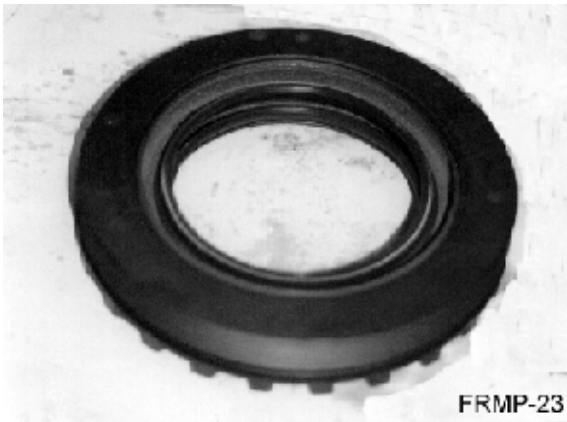
Picture 33: Input shaft bearing adjustment nut with its seal.
