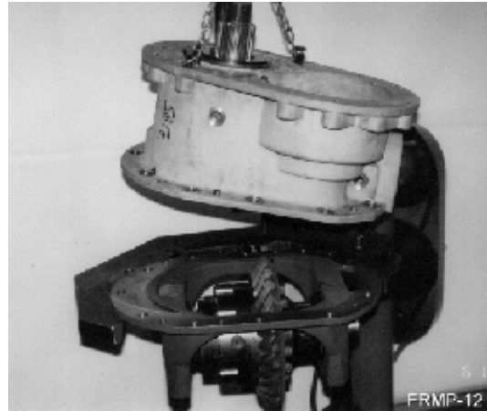
Picture 14: Removal of the spur gear housing
