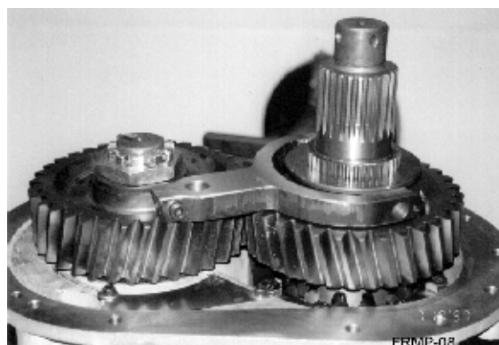
Picture 10: Housing and bearing removed; differential lock fork still in position.
