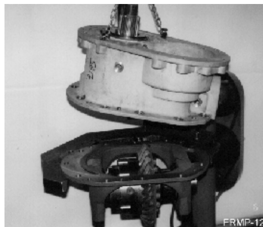
Picture 20: Installing of the spur gear housing
