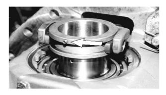
Picture 6. Sliding ring lock screw loosened (arrow).
