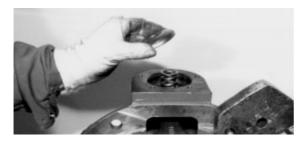
Picture 3. Support cup and spring ready for removal.
