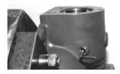
**Picture 4.** Allen wrench in fork lock screw access hole.
