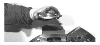
**Picture 2.** Lock cylinder cover removed and diaphragm is loose.
