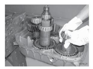
Lift out intermediate shafts and output shaft.
