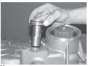
Install shifting piston with seal.
