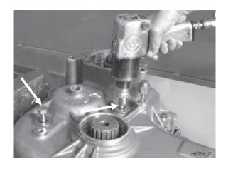
Disassemble anchor screws.
