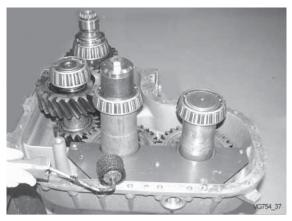
Apply LOCTITE 518 on front housing.
