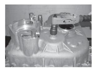
Check rolling torque of the double gear.
