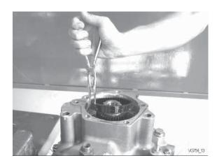
Slide outer pump gear on oil pump gear.
