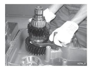
Mount input shaft together with shift fork and shift rod.
