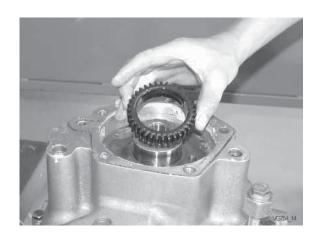
Remove oil pump gear.
