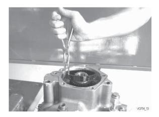
Remove outer oil pump gear.
