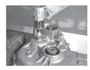
Disassemble oil tube.
