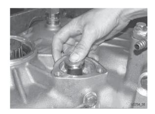
Slide cylinder and seal on shift rod.
