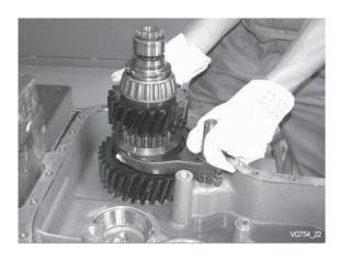
Install input shaft together with shifting fork and shift rod.
