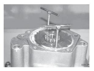
Lift off oil pump housing.
