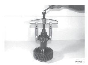
Pull off the rear tapered roller bearing.
