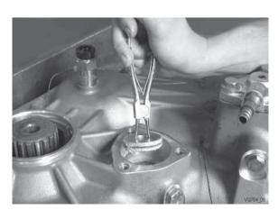
Pull off piston with sealing.
