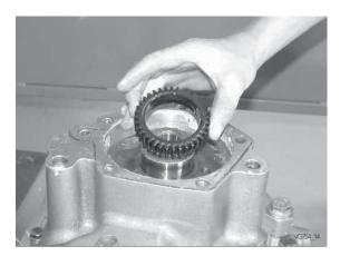
Install oil pump gear on input shaft.
