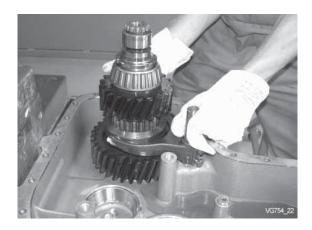
Lift out input shaft together with shifting.
