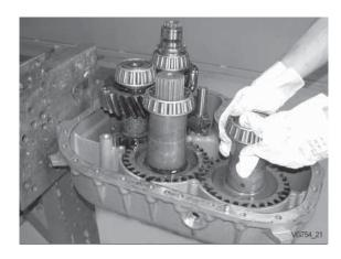
Install intermediate shafts and output shaft.
