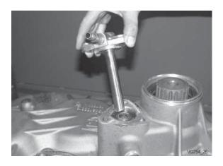
Remove cover and shifting shaft together.
