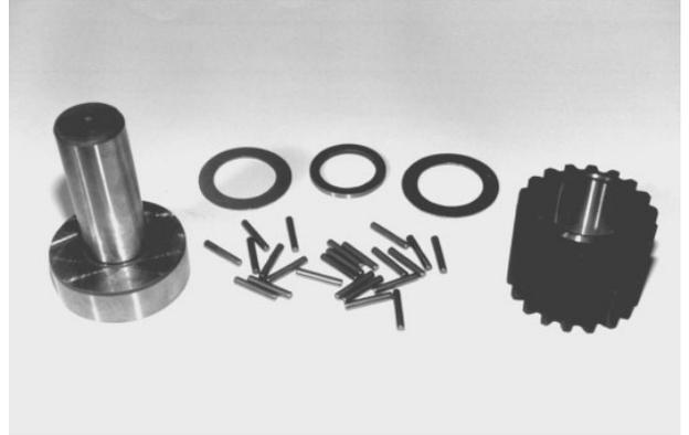
**Picture 5. Parts of one planetary gear** (some bearing needles missing)
