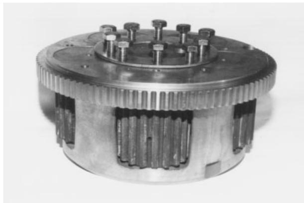
**Picture 4. Planet gear shaft lock screws loosened.**
