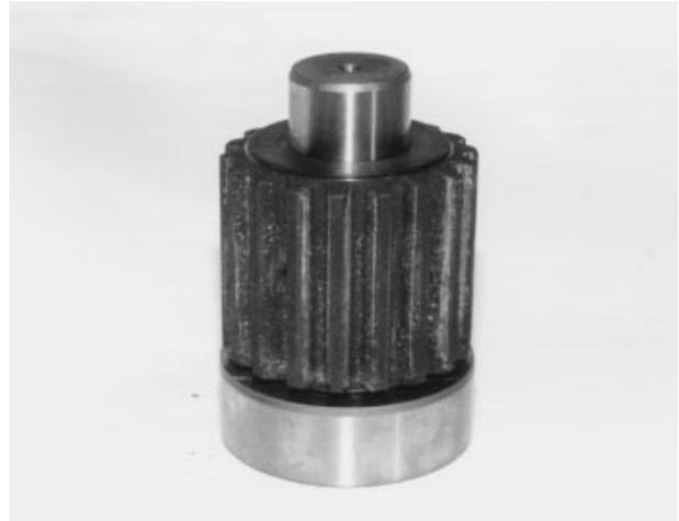
**Picture 7. Planet gear with planet gear shaft in place ready for installation in planetary carrier.**
