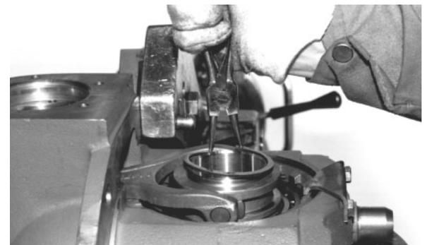
**Picture 7.** Removing sliding ring snap ring.
