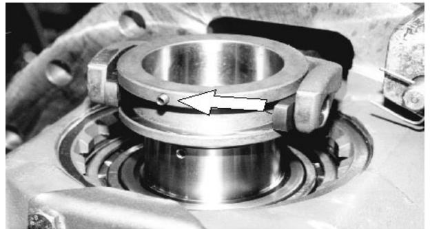
**Picture 6.** Sliding ring lock screw loosened (arrow).
