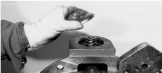
**Picture 3.** Support cup and spring ready for removal.
