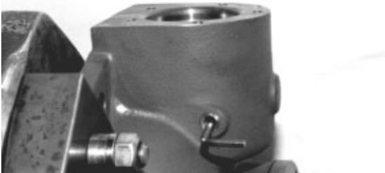
**Picture 4.** Allen wrench in fork lock screw access hole.
