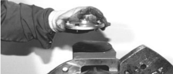
**Picture 2.** . Lock cylinder cover removed and diaphragm is loose.
